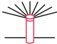
They have a lower application rate, which reduces runoff from compacted clay soils and slopes.
