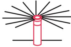
Pop-up spray heads have a high water delivery rate of 1-2 ½ inches per hour. At the typical rate of 1 ½ inches per hour, the zone would receive a half inch of water in just 20 minutes.
