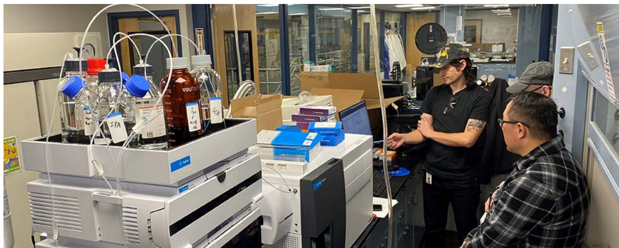
Image 16. Thornton Water Quality Analysts setting up a new LC/MS instrument for measuring PFAS.
